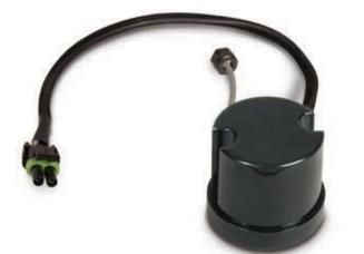
The PQS is a bi-directional current limit control. The control monitors current during actuator motion and quickly stops the actuator if an object gets in the way or at the end of stroke. The actuator will remain off until power is reapplied. The current limit setting is adjustable with two potentiometers that are accessible through two plugged holes on the side of the housing.
